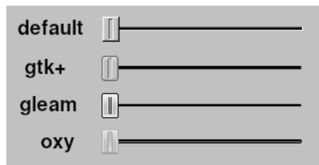
Figure 12.25 FI_Hor_Nice_Slider with various FI::scheme() values
